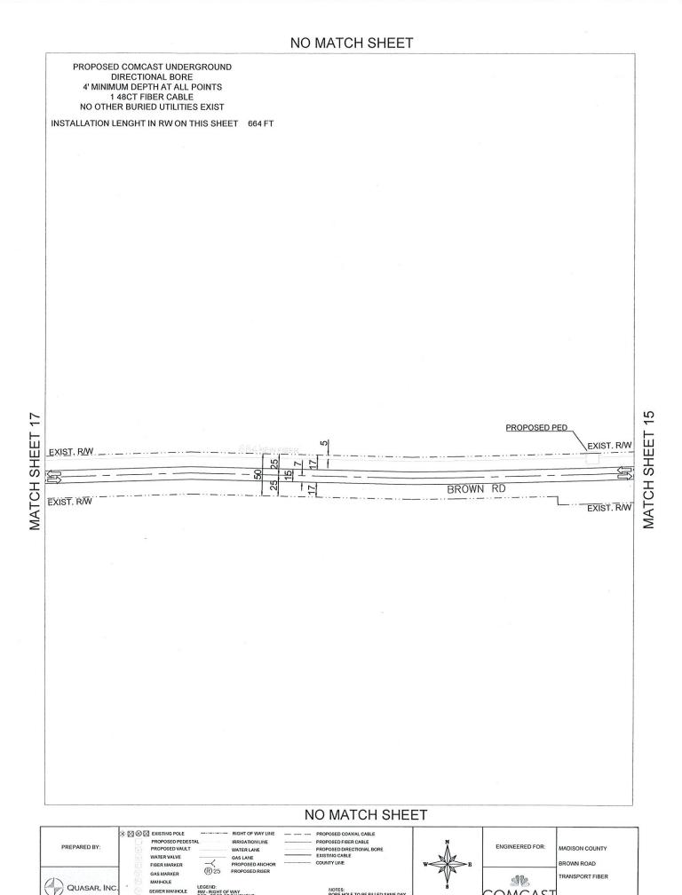
NOTES: BORE HOLE TO BE FILLED SAME DAY VAULT HOLE TO BE FILLED SAME DAY ALL HOLE TO BE TAMPED AND SODDE
