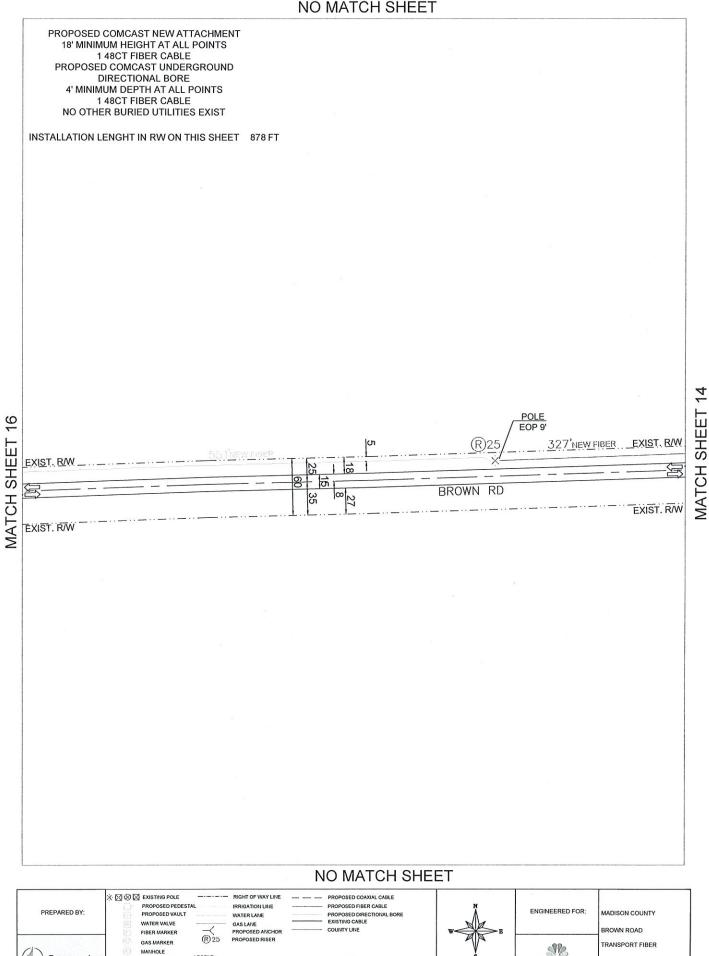
NOTES: BORE HOLE TO BE FILLED SAME DAY VAULT HOLE TO BE FILLED SAME DA' ALL HOLE TO BE TAMPED AND SODD
