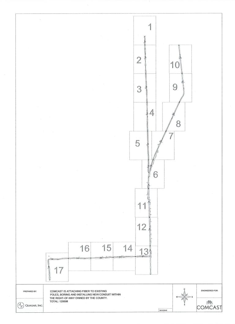
PROPOSED COMCAST UNDERGROUND DIRECTIONAL BORE 4' MINIMUM DEPTH AT ALL POINTS **1 24CT FIBER CABLE** NO OTHER BURIED UTILITIES EXIST
